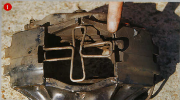
This is a front caliper from our 964-model 911 Carrera 4. The stainless-steel plate on the left of the photo has clearly lifted away from the aluminium caliper body beneath. It would be impossible to fit new brake pads in this situation without grinding material from the pads' backing plates – which certainly isn't recommended
