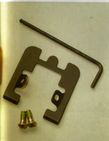
Repair kit consists of plate and two special screws – you'll need four kits per car
