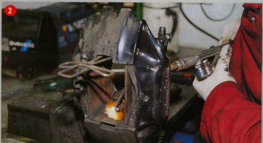
Once you've removed the brake pads you need to undo the two screws holding each plate in place. They're secured with thread-locking compound, so you'll have to heat them in order to release them. Protect the pistons and their rubber seals with steel plates (cut roughly to the size of the brake pads) and direct a blowtorch on the screw head until it's red-hot. You can then remove it with a 4mm hexagonal key (or possibly a Torx driver if the screw has been renewed before; more on this in a moment)
