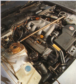
Overbored block and 52 crankshaft give engine capacity of 2.8 litres. Internal mods improve piston cooling and oil return
