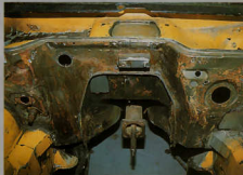
The holes where the heater pipes pass through the front bulkhead are blocked with aluminium sheet and sealant to create the required safety wall between the engine compartment and the cockpit
