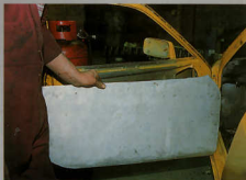
Door cards and side-trim panels are replaced with aluminium sheet cut to size using the originals as templates and then riveted in place. The window operating system is removed to reduce weight
