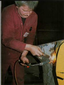
Kevin Eacock gets to work scraping the under-body sealant and sound-deadening material from the shell. It's a messy and time-consuming job, but makes it easier to achieve the minimum weight limit of 1100kg
