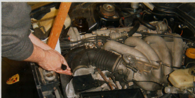
Removing the standard air flow meter. Note Bennett's optional wooden bonnet stay. One day, he'll change the struts!
