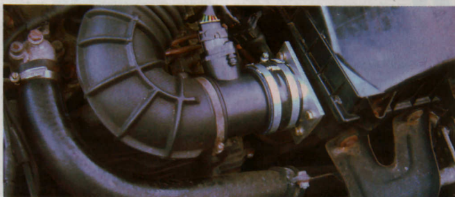
ProMax MAF kit in place. Note how it's a straight replacement for the standard air flow meter. Below: on the rollers
