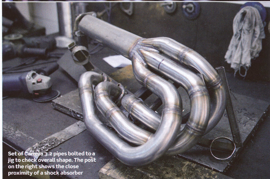
Stainless steel is a mild steel alloy with chrome content, plus nickel and zinc. H&S uses mainly BS304 or BS316 tubing, which contains 18 per cent chrome, with a wall thickness of 1.2 or 1.6mm
