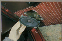
Speakers and grilles are secured by four screws. Don't lose plastic spacers
