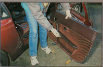
Inner door trim comes off with armrest – but not lower pocket – still attached
