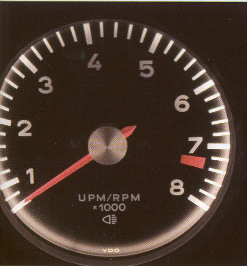
Above: Prototipo steering wheel is an original fitment, as is the Carrera-spec tachometer, with its 7300rpm red line. Maximum power was produced at 6300rpm, but an extra 1000rpm allowed full use to be made of the gear ratios. Interior trim is funeral black
