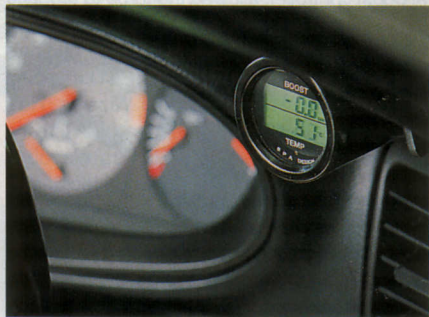
Digital boost gauge and engine-oil-temperature gauge (above) sit neatly on the edge of the dashboard. Interior (below) is otherwise standard 944 fare
