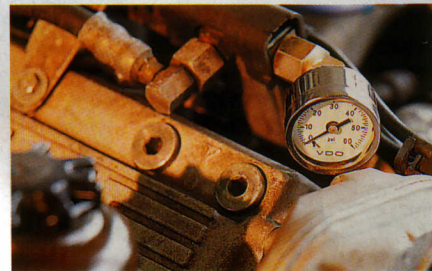
Neat gauge (above) at the end of the fuel rail indicates fuel pressure at this point. Engine (below) looks standard apart from pipework to the turbocharger
